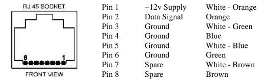
Pins 5, 6, 7, & 8 are not required but if you are using standard CAT 5 cable you can terminate the spare wires to keep the cable tidy.
